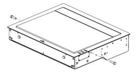
Remove the 2 front transport plastic screws M8x30
